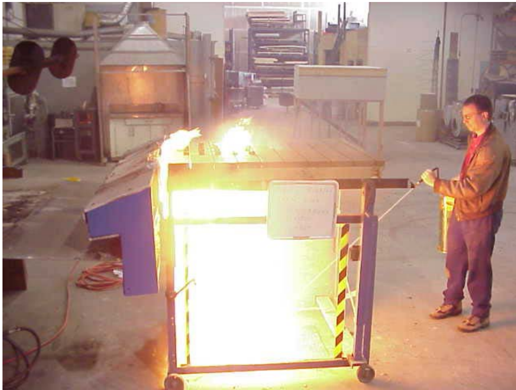
Figure 4. Plastic lumber fire propagation test after 29 minutes.
